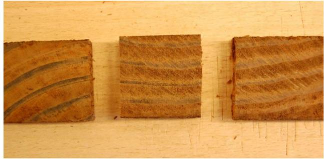
**Figure B2:** Test pieces with parallel growth rings
